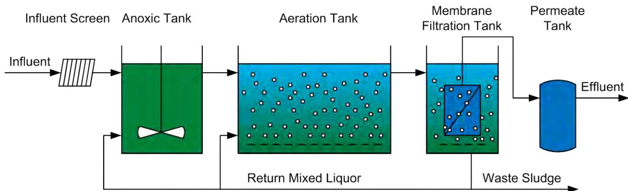
**Figure 2. MBR Process Schematic Diagram**
