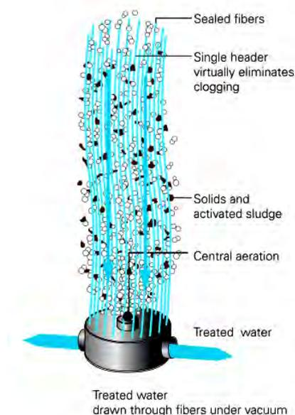
**Figure 3. Single Header Hollow Fiber Membrane**
