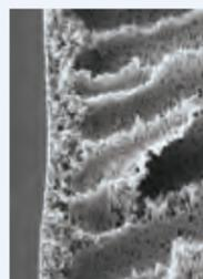
MicroClear ultrafiltration membranes are asymmetric – featuring smaller pores on the raw water side than the permeate side. This ensures that viruses and microscope particles are retained, while minimizing pressure loss inside the membrane.
