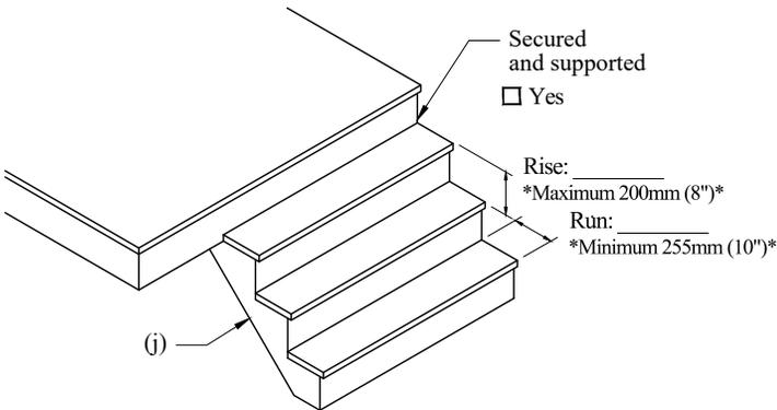
**NOTE:** Handrail required when more than 3 risers.
